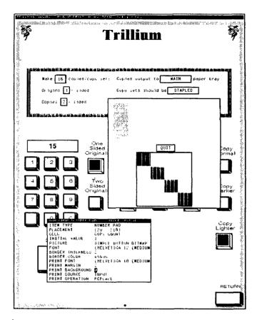
Figure 2: A portion of the Trillium screen containing an editor for a NumberPad showing its characteristics and their values, and a shade editor being used to modify one of those values.
